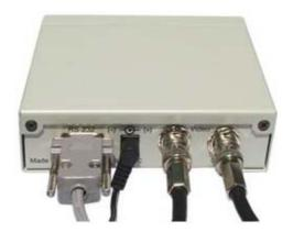
Serial Input Power Video Input Video Output
