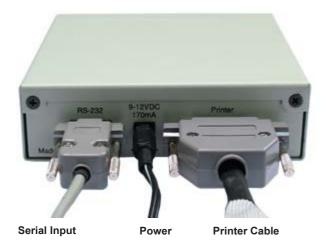
Figure 3B: P2RS Parallel-to-Serial Converter
